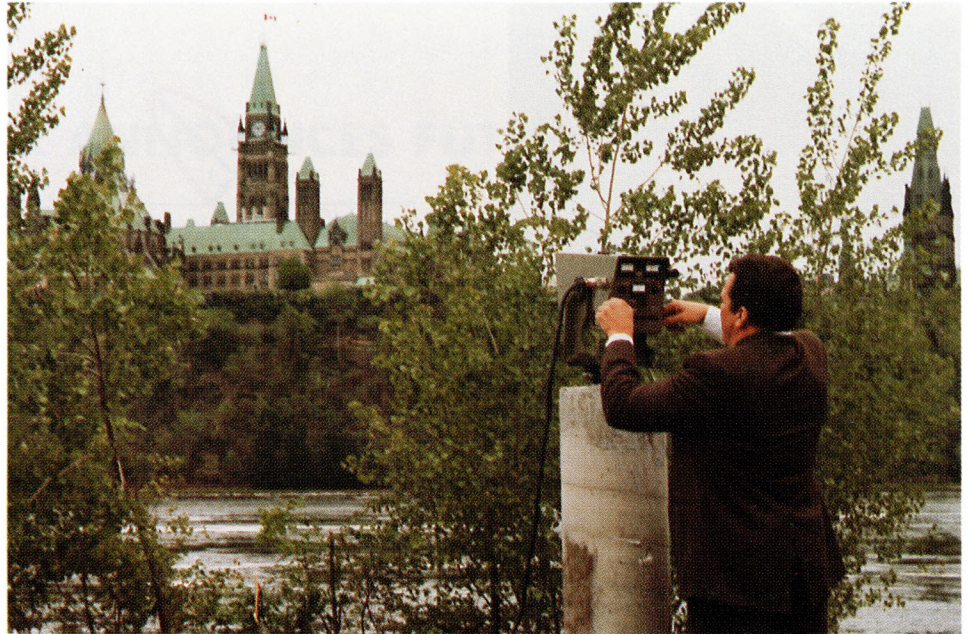
Figure 4. ME 3000 instrument used to measure distances with submillimetre precision.
