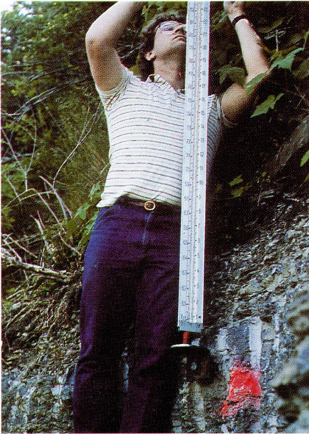
Figure 6. Precise geometric leveling was done to determine the heights of the control and monitoring stations.
